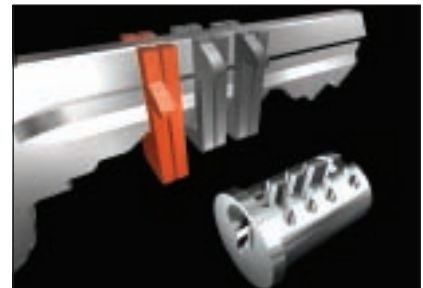
There are 10 CYL4™ wafers numbered 0-9, that cover the 10 depths of a C4 key. Six wafers are arranged in pairs to match the first 3 cuts of the customer's key.
