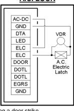
\* Use 1N4004 diode only when using a door strike not a Magnetic Lock or Drop Bolt.
