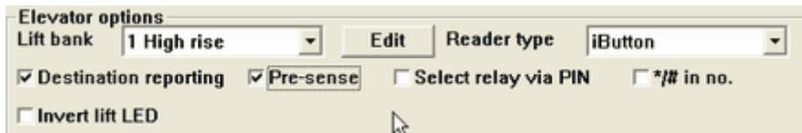
With the 'destination reporting' box ticked, when a credential is used in the lift no transaction will be reported until either a floor is selected or the trigger time elapses. If the 'pre-sense' box is ticked then the relays themselves will not operate until the floor destination inputs detect a floor being selected in the elevator.
