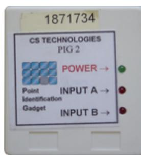
The PIG-2 connects to the PIG-bus either directly to the controller or in a daisy-chain to the previous PIG in the bus. Up to 25 PIGs may be connected to a single bus. It is recommended that a PIG-booster also be fitted to ensure reliable communication with the PIGs.
