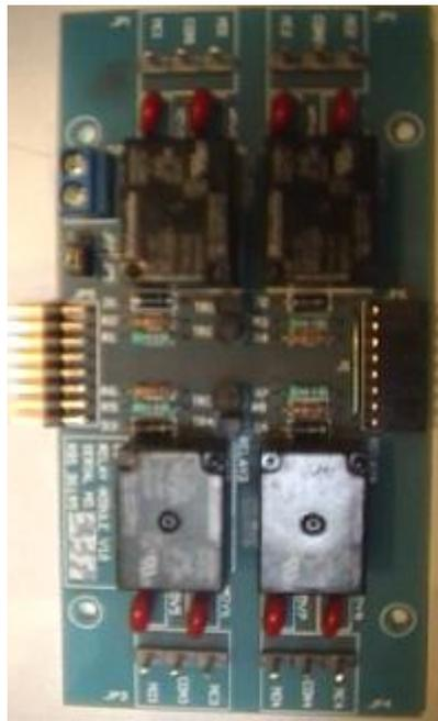
The 4-way relay board connects to the expansion port of the controller via a ribbon cable. Additional 4-way relay boards connect to the first one via the 16-way header on the edge of the board. A diagram of the 4-way relay board is below.
