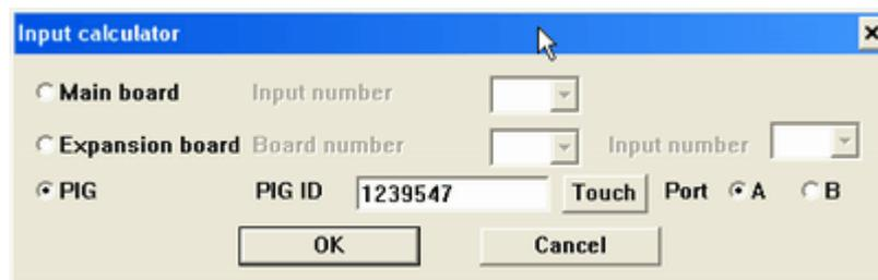
If the input is on a PIG the ID can be entered, and port A or B selected. In this case a PIG has been selected for the input, and port A will be used.
